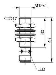
Inductive Sensors BES 516-375-E5-C-S 4 M12x1 x 45 normally-closed Sn=2mm shielded
